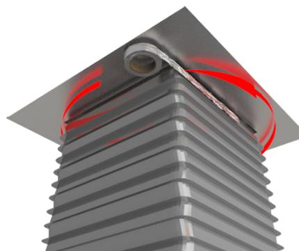
Using aluminium tape provided, secure flexi shaft to zincolume shroud at bottom of roof assembly.
