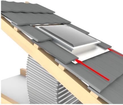
Slide the soaker tray up under the top and side tiles and over the bottom tiles.
