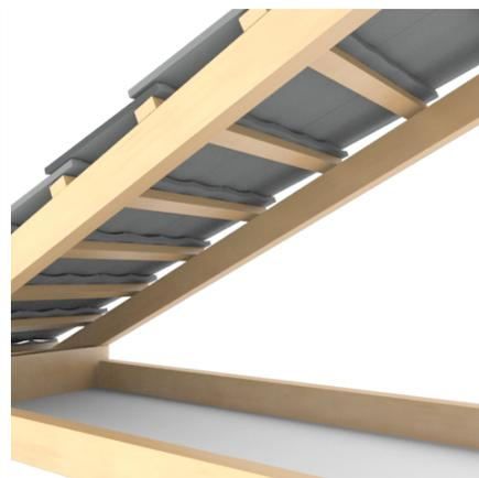
Decide location for skylight by inspecting inside roof cavity for obstructions such as hanging beams, under purlins, etc. Whenever possible, locate the ceiling ring directly below the roof assembly. Also, try to locate one edge of ceiling frame next to joist/truss.
