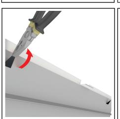
Attach flexi shaft to alumium shroud by peircing the tabs through the shaft and folding upward with pliers.
