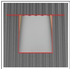
Using jigsaw, cut out marked lines and remove square roof sheet peice.
