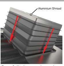
Carefully lower shroud and flexi shaft through the opening in the soaker tray.
