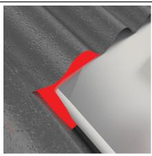
Backfill extended cuts at top corners of soaker tray with silicone.
