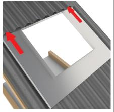
Lifting the top edge cut, slide the soaker tray up and under the cut. Rest the soaker tray on the roof sheeting. Secure the soaker into position using tech screws provided. Tech screws must be sealed with silicone.
