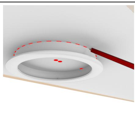
From ground level (looking up at ceiling) locate the original hole for positioning ceiling ring. Hold ceiling ring to ceiling with hole in dead centre. Trace the outside of the collar with a marker.
