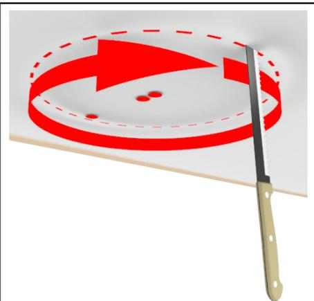
Using a plaster knife or jigsaw, cut out the plaster circle and remove.
