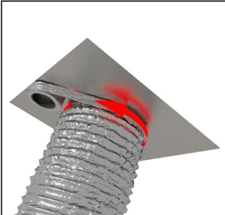
Fix the flexi shaft to the collar on the underside of the dome using the aluminium tape provided.
