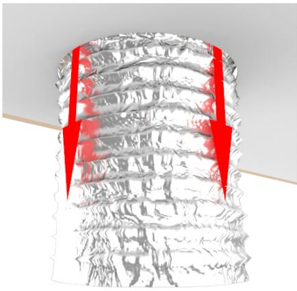
Pull excess flexi shaft through hole in ceiling.
