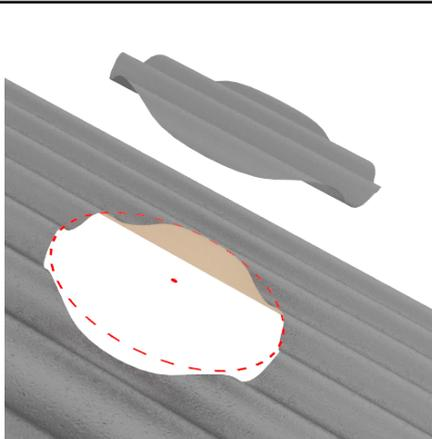
Using a jigsaw or tinsnips, cut a circle in the roofing sheet 10mm larger than the flexi shaft diameter.
